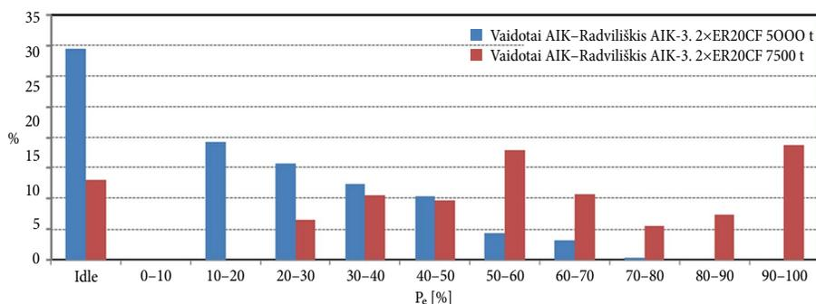
Fig. 4. Operational load cycle structure of the 2ER20CF locomotive diesel engine on the line Vaidotai–Radviliškis (train weight 5000 t and 7500 t)
