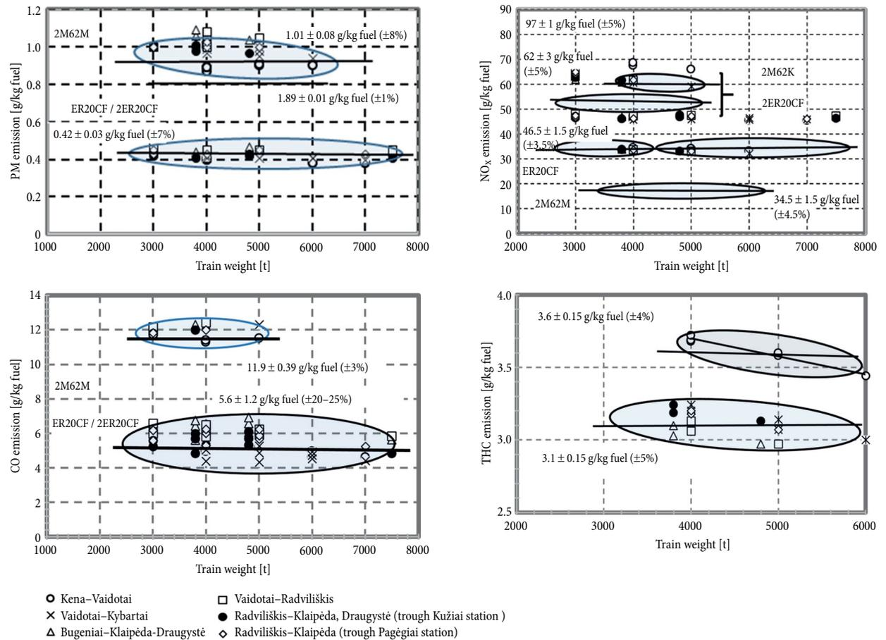
Fig. 3. Ecology indicators of diesel engines of freight locomotives (HCSE [g/kWh]) operated by the JSC ‘Lithuanian Railways’
