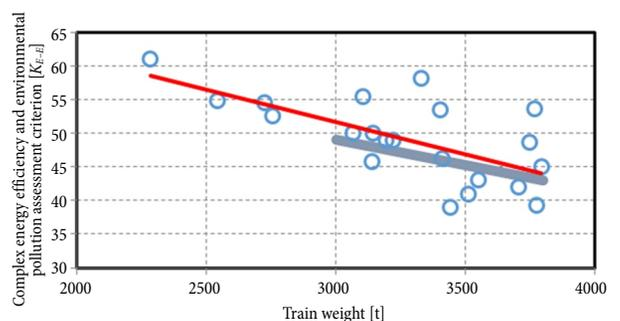
Fig. 7. Theoretical and actual values of complex  $K_{E-E}$  criteria values of a single section locomotive ER20CF on the railway line Radviliškis–Draugystė: o – operational experimental points; — — theoretical trend; — — actual data trend
