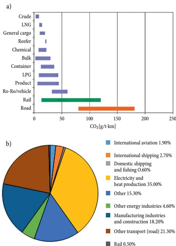
Fig. 1. Specific CO<sub>2</sub> emissions [g/t·km] (a) and CO<sub>2</sub> emissions [%] from vehicles in the overall global balance (b) (IMO 2009)
