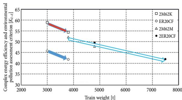
Fig. 5. Evaluation of energy efficiency on freight transportation line Bugeniai–Klaipėda/Draugystė
