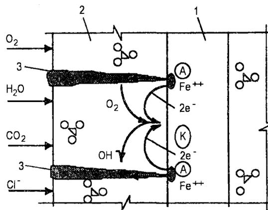
**Fig 1.** Scheme of reinforcement corrosion in concrete:
