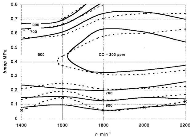
Fig 3. Dependency of carbon monoxides CO emission on engine revolution frequency ( $n$ ) and load ( $bmep$ )
