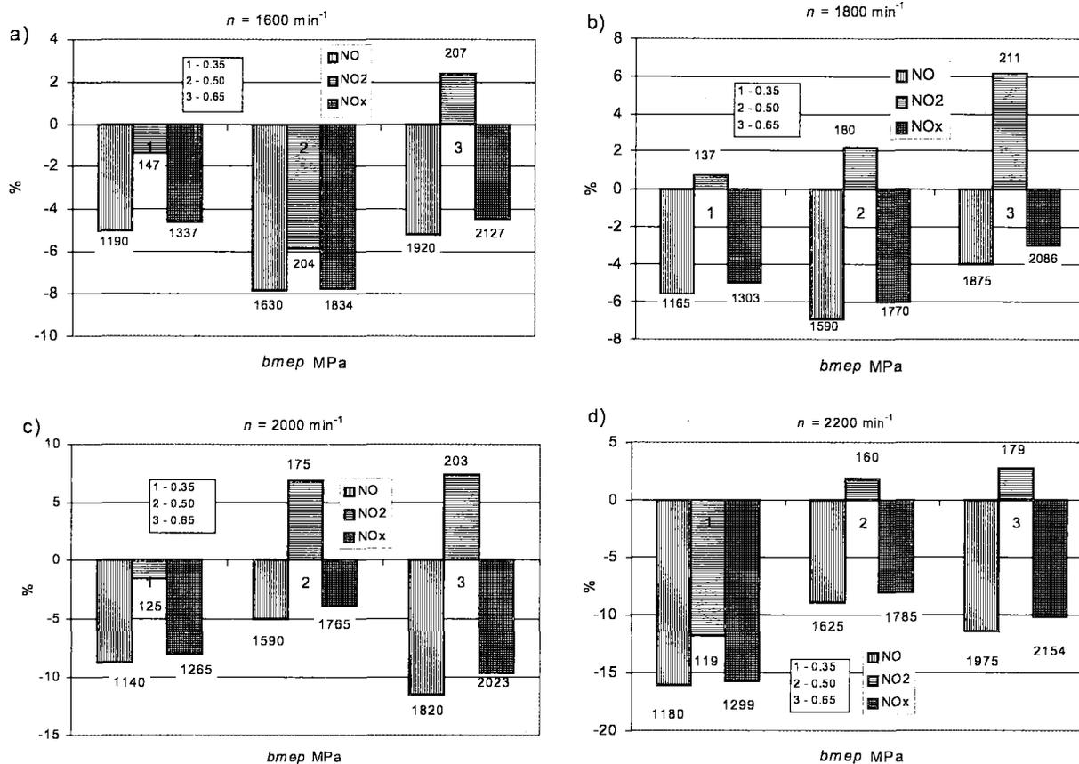
Fig 2. Influence of fuel additives SO-2E on nitrogen oxides NO, NO<sub>2</sub> and NO<sub>x</sub> emission when running the engine at different loads  $bmep = 0,35; 0,50$  and  $0,65$  MPa and various revolution frequencies  $n = 1600$  (a);  $1800$  (b);  $2000$  (c) and  $2200$  (d)  $min^{-1}$
