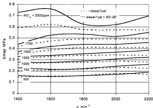
Fig 1. Dependency of common nitrogen oxides  $\text{NO}_x$  emission on engine revolution frequency ( $n$ ) and load ( $b\text{mep}$ )
