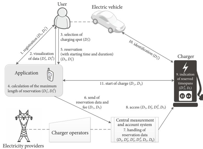
Figure 3. Model of “Charging spot reservation” function
