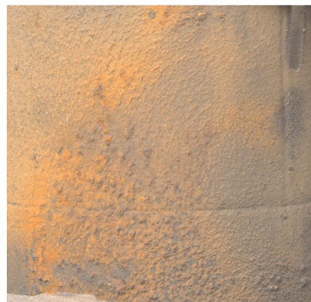
Fig 1. Scale deposit on the cylinder surface
