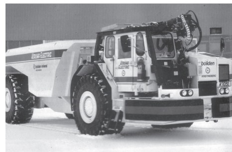
Fig 2. Haulage truck supplied by contact lines in a mine
