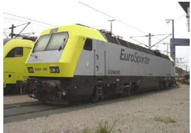
Fig. 12. Electric AC locomotive class EuroSprinter
