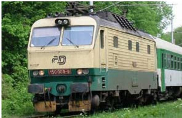
Fig. 10. Electric DC locomotive Skoda class 150
