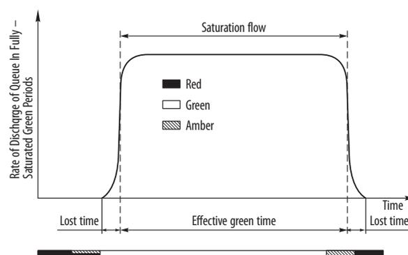
Fig. 1. An idealised model of saturation flow
