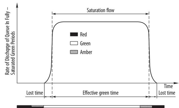
Fig. 1. An idealised model of saturation flow
