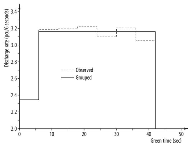
Fig. 5. Discharge rate for site n°3 per 6-second interval
