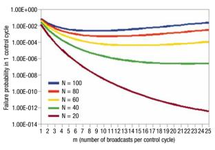
Fig. 8. The probability of communication failure in one control cycle
