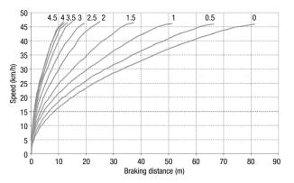
Fig. 6. Relationship between speed and braking distance for different values of braking pressure (in volts applied to the electro-proportional pilot)
