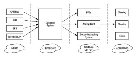
Fig. 1. The structure of controlling AUTOPIA system
