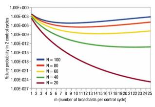
Fig. 9. The probability of communication failure in two control cycles
