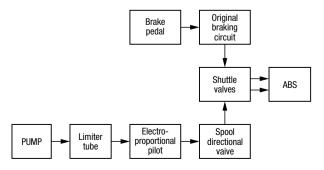
Fig. 3. The design of the electro-hydraulic braking system
