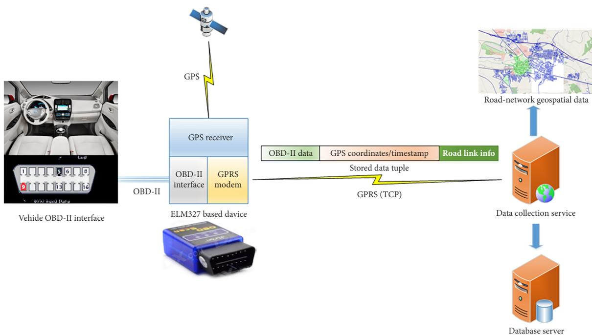
Figure 2. Experimental data collection setup
