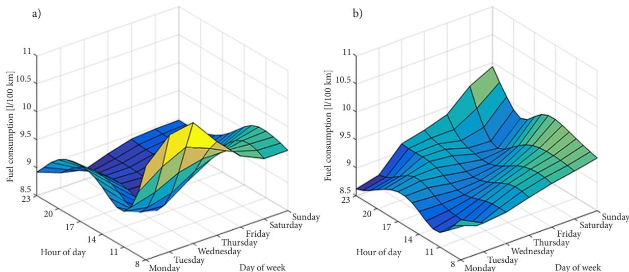
Figure 7. Passenger car fuel consumption in the city of Niš during winter: a – Zone 1; b – Zone 2
