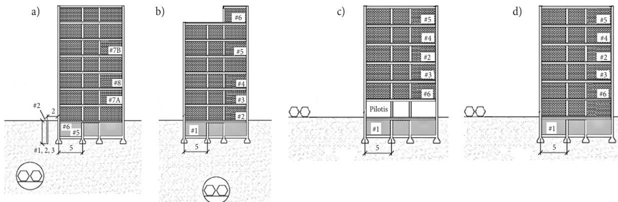
Fig. 1. Cross-section of the: a – PPC building and measurement locations; b – Mourouzi street building; c – Maroussi 1 building; d – Maroussi 2 building
