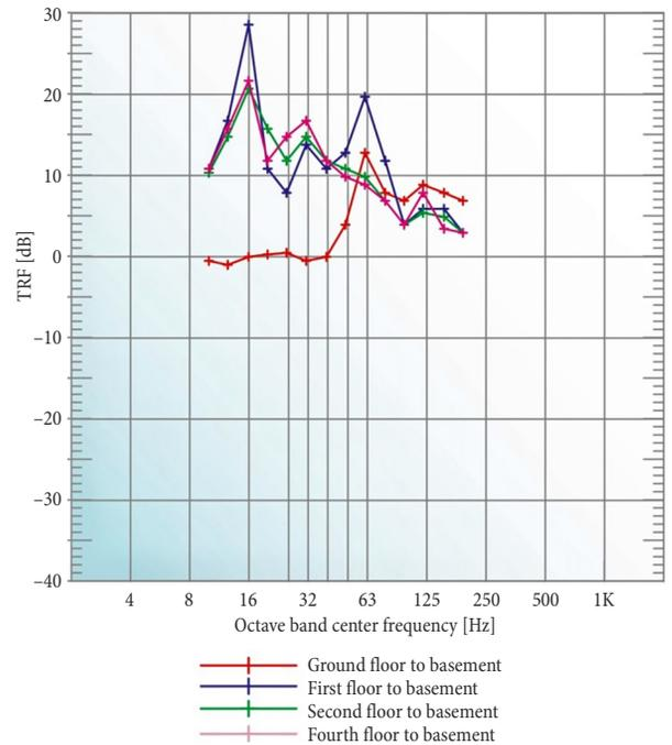
Fig. 8. Average amplification factors relative to PPC building basement
