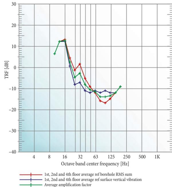
Fig. 6. Average amplification factor at PPC building for 1st, 2nd and 4th floor data
