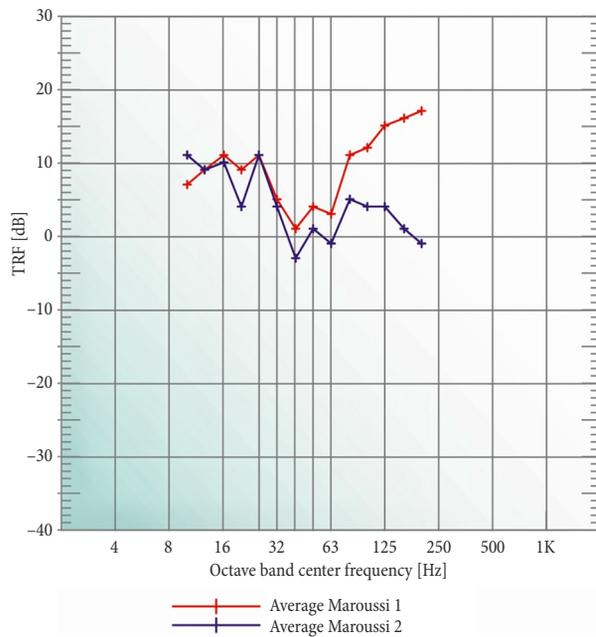
Fig. 12. Average 1st floor to basement relative vertical vibration levels for Maroussi 1 and Maroussi 2 buildings
