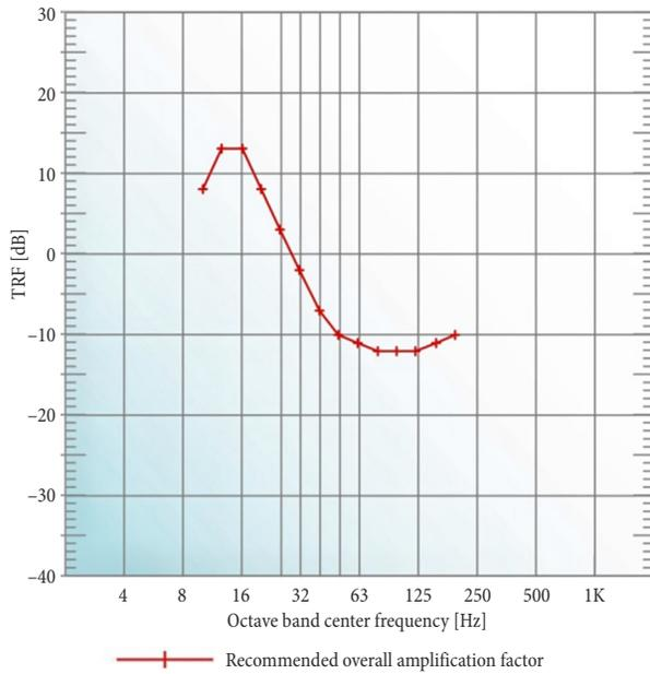
Fig. 7. Recommended amplification for occupied floors of typical buildings in Athens
