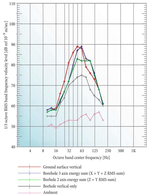
Fig. 2. Borehole and surface averages for sets A and B train vibration in the borehole and at the ground surface
