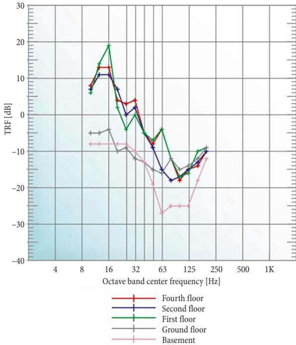
Fig. 3. Average amplification factors relative to borehole Root Mean Square (RMS) sum vibration levels
