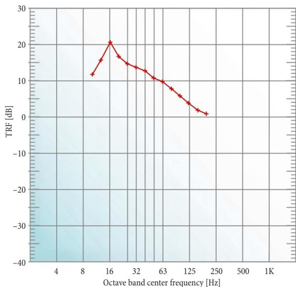
Fig. 10. Recommended amplification factors from basement to upper floors in PPC building
