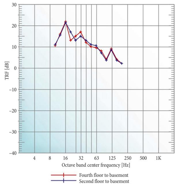
Fig. 9. Average amplification factors from basement to upper floors in PPC building
