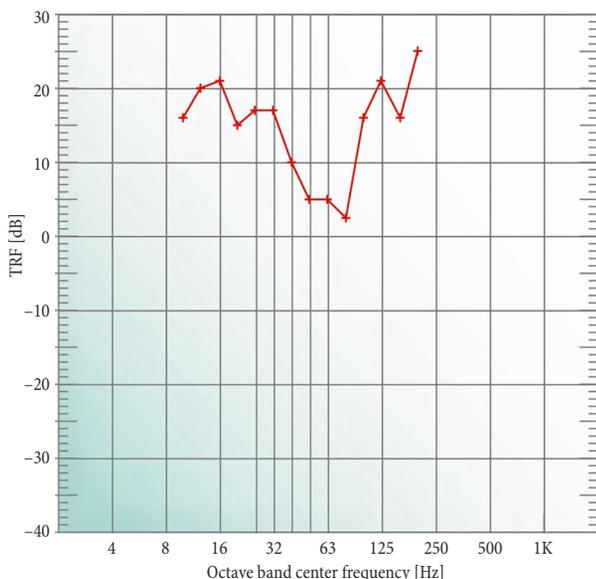
Fig. 11. Mourouzi street building: transfer function from the basement to the 1st floor
