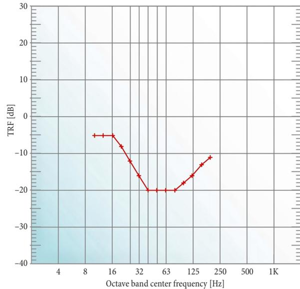
Fig. 5. Recommended coupling loss between soil and basement
