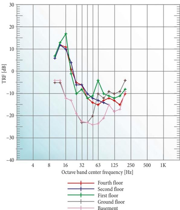
Fig. 4. Average amplification factors relative to surface vertical vibration levels
