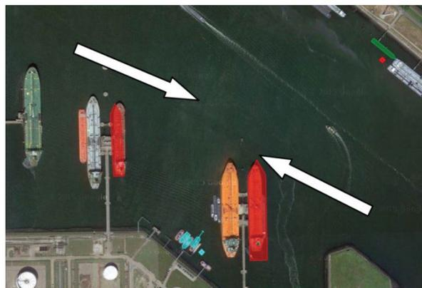
Fig. 2. Jetties for the oil terminal at the Port of Rotterdam and directions of tidal currents
