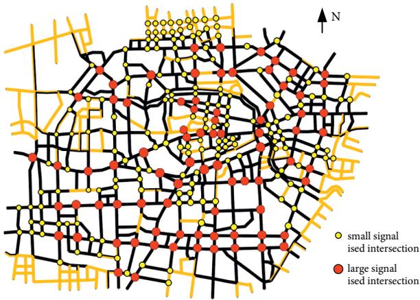
**Figure 7.** Initial partition based on MST (the black road network is the largest sub-tree, and the rest of the scattered sub-trees are marked as yellow)
