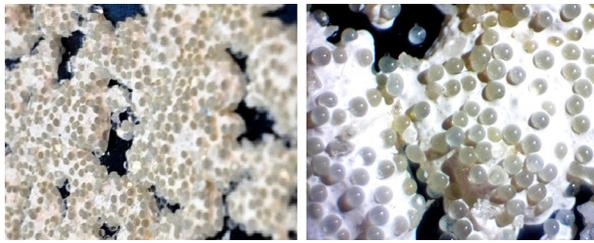
Figure 3. Illustration of a cold plastic structural marking (laboratory sample)
