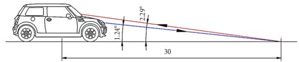
Figure 2. Illustration of the principle of night-time visibility measurement, illustration is not in scale (source: adapted by authors)
