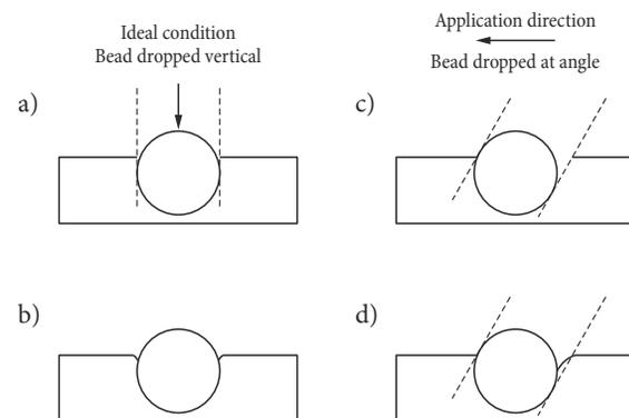
Figure 1. Different bead embedment illustration (Rasdorf *et al.* 2009)
