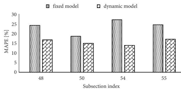
Figure 11. MAPE comparison between fixed and dynamic models in rainy days
