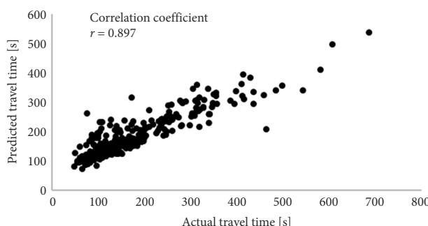
Figure 5. Sample scatter plot of actual vs. predicted travel times (temporal SVM)
