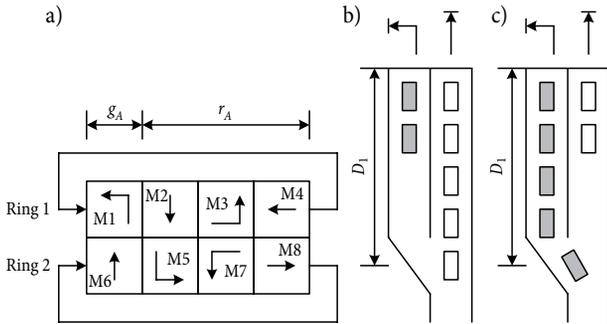
Fig. 3. Blockage and overflow of short left-turn lane under left-through phasing: a – signal phase sequence; b – blockage of short left-turn lane during the red phase for both left-turn and through movements; c – overflow of short left-turn lane during the red phase for both left-turn and through movements
