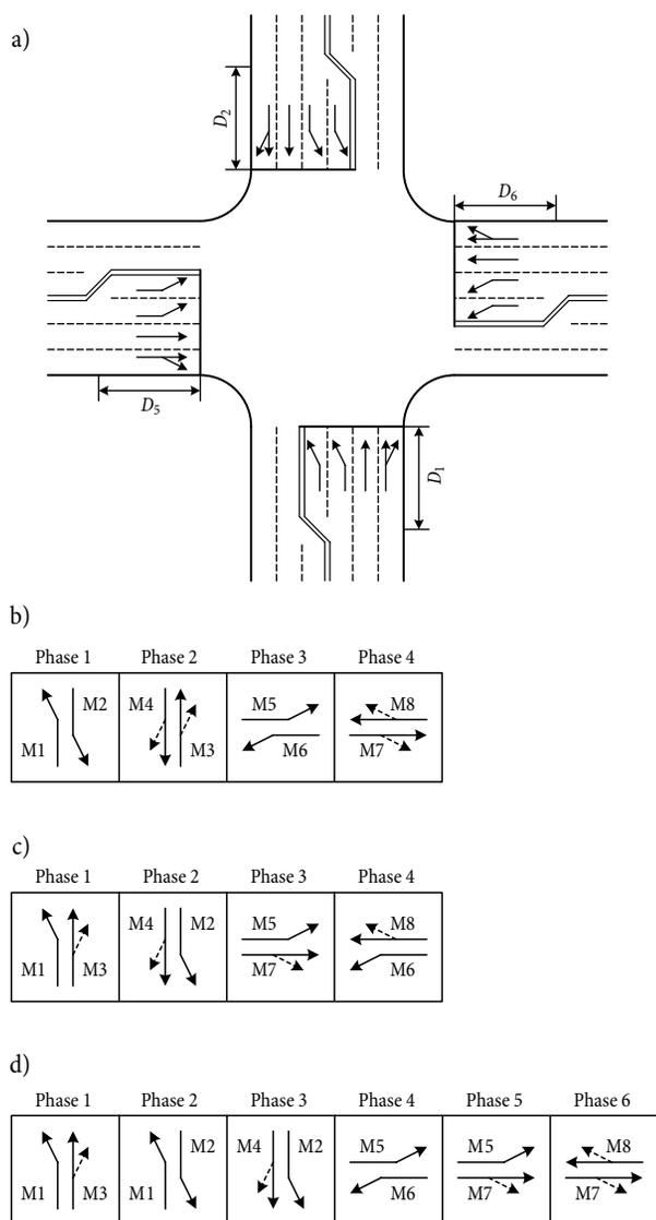
Fig. 5. Channelization scheme and signal phase plans for a four-leg intersection: a – channelization scheme; b – exclusive left-turn phasing; c – left-through phasing; d – overlapping phasing
