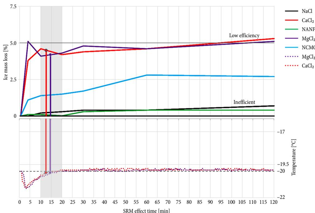
Fig. 3. Loss of ice mass and the change in surface temperature ( $t = -20\text{ }^{\circ}\text{C}$ ) (Bulevičius et al. 2014)
