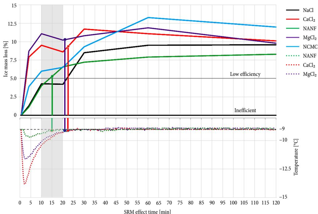
Fig. 2. Loss of ice mass and the change in surface temperature ( $t = -9^{\circ}\text{C}$ ) (Bulevičius *et al.* 2014)
