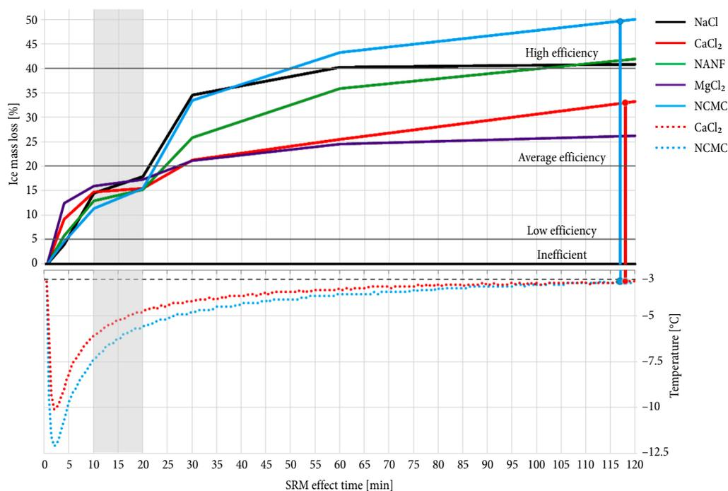
Fig. 1. Loss of ice mass and the change in surface temperature ( $t = -3\text{ }^{\circ}\text{C}$ ) (Bulevičius *et al.* 2014)
