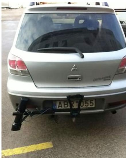
Fig. 4. Sensor for measurement of friction (RCM 411) installed on a tow-ball of a vehicle (Bulevičius *et al.* 2014)
