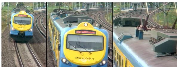
Fig. 8. Set of three camera images taken, for identification of vehicle and raised pantograph
