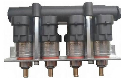
Fig. 3. Subject of the research – a system of injectors
