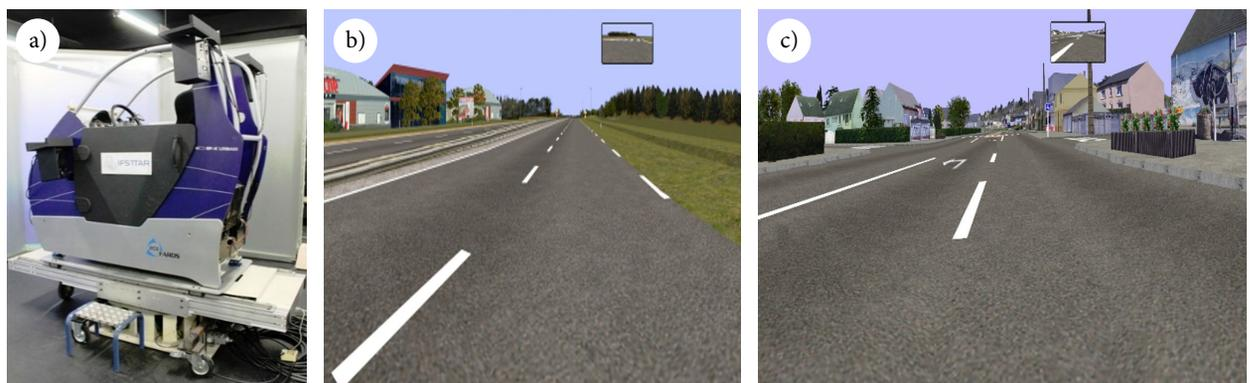
Fig. 4. Two DoF driving simulator (a), virtual environment (b, c)
