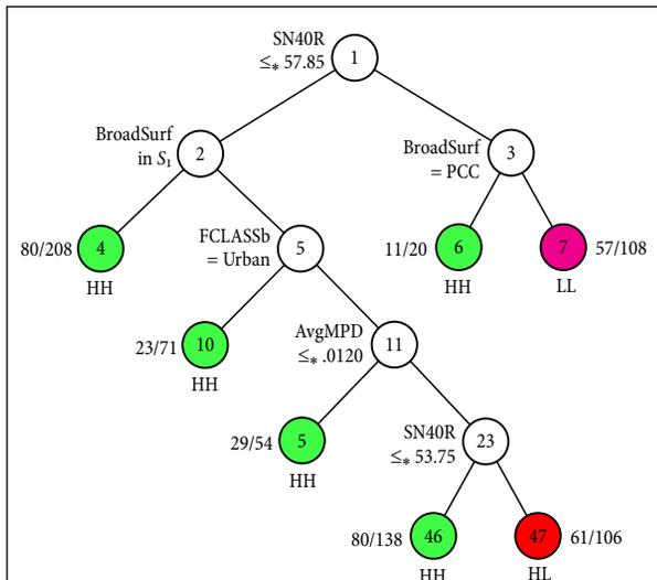
GUIDE classification tree with estimated priors and unit misclassification costs. At each intermediate node, an observation goes to the left branch if and only if the condition is satisfied. The symbol '≤' denotes '≤ or missing'. Set  $S_1 = \{PCC, SMA\}$ . Predicted classes (based on estimated misclassification cost) below terminal nodes; #misclassified/sample size beside each node.
