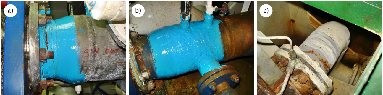
Figure 9. Repair pipe SW (sea water) line for cooling LT (low temperature) contour by comp. materials as Wet Wrap technology of container ship MERWE TRADER (in this case, fiberglass impregnated with compositions based on modified epoxy resins was used)
