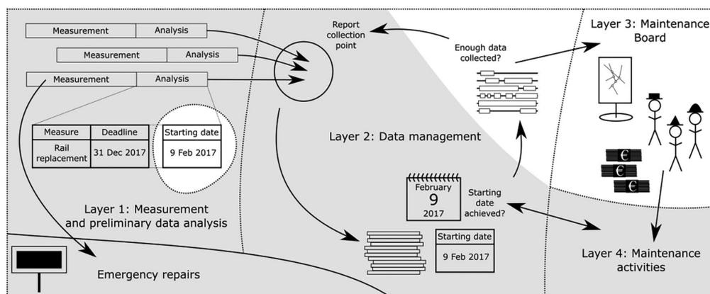
Figure 2. Framework of the infrastructure maintenance process – based on research by Smoczyński (2018)
