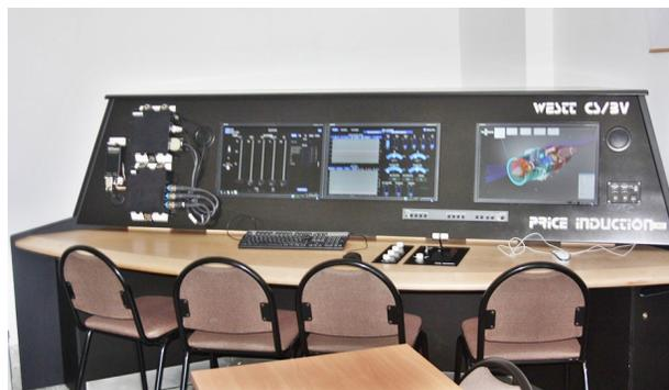
Figure 5. Virtual engine test bench WESTT CS/BV, the measurement data is displayed on the screens
