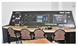
Figure 5. Virtual engine test bench WESTT CS/BV, the measurement data is displayed on the screens
