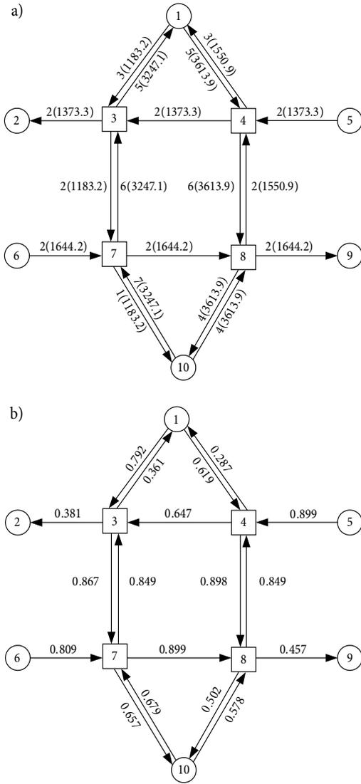
Fig. 4. The solutions for network capacity problem with Strategy 1: a – optimal link flow solutions (in brackets) and number of lanes (out of brackets) for network capacity problem with strategy 1; b – the Volume/Capacity (V/C) of each link at maximum network capacity state of Strategy 1
