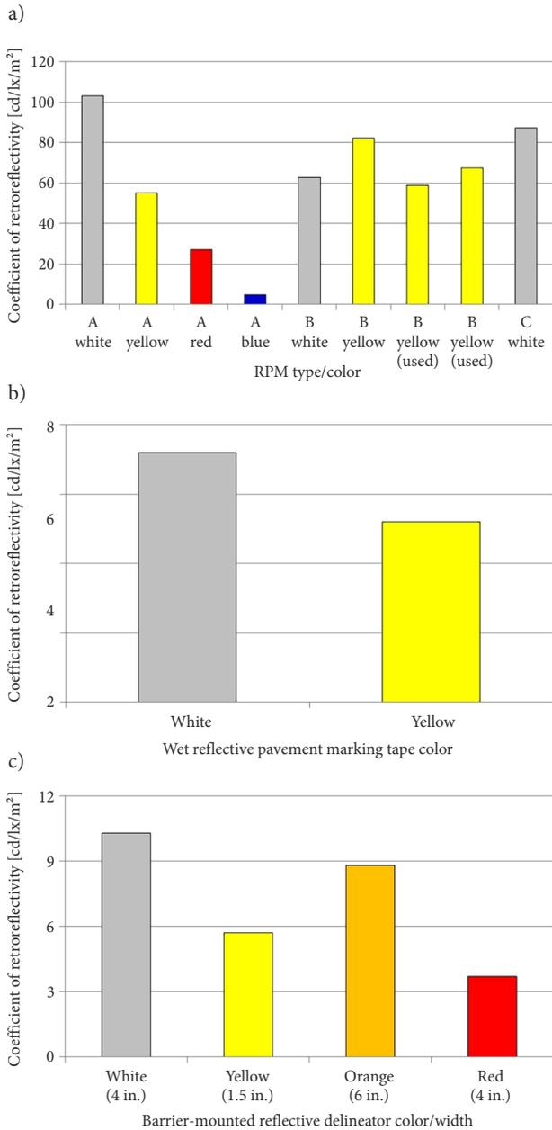
Figure 7. Coefficients of retroreflectivity [cd/lx/m<sup>2</sup>] for: a – RPMs; b – wet reflective pavement marking tape; c – barrier-mounted reflective delineators
