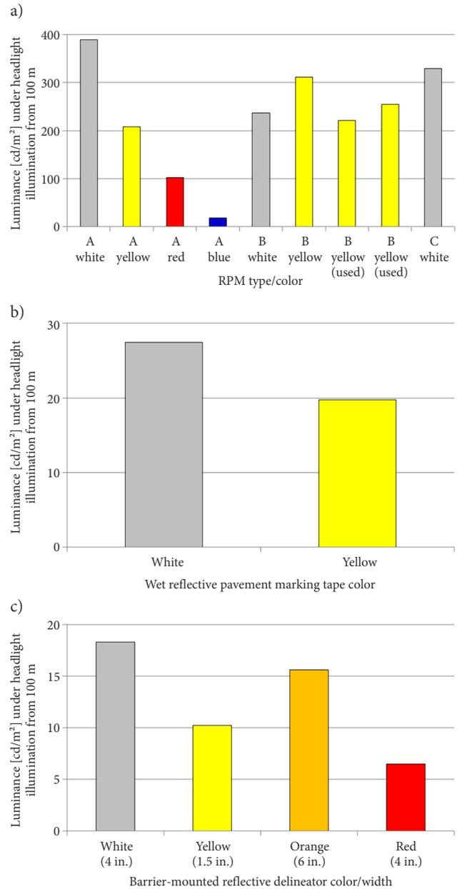
Figure 8. Luminances [cd/m<sup>2</sup>] under headlight illumination from 100 m away for: a – RPMs; b – wet reflective pavement marking tape; c – barrier-mounted reflective delineators
