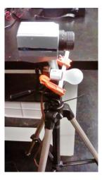
Figure 4. Luminance meter and light source (left: front view, right: side view)
