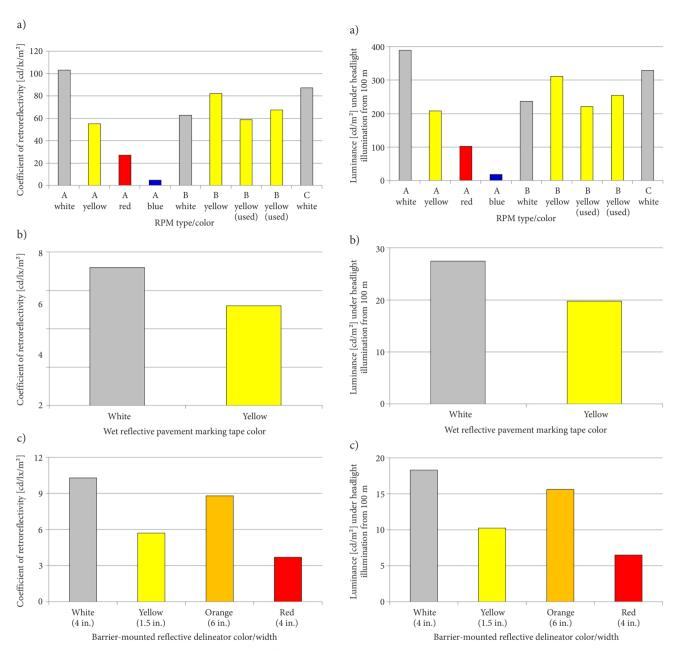
Figure 7. Coefficients of retroreflectivity [cd/lx/m²] for: a – RPMs; b – wet reflective pavement marking tape; c – barrier-mounted reflective delineators
