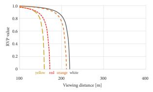
Figure 12. RVP values for each barrier-mounted reflective delineator color, as a function of viewing distance
