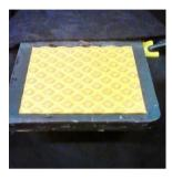
Figure 2. Examples of wet reflective pavement marking tape samples
