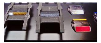
Figure 1. Examples of RPM samples
