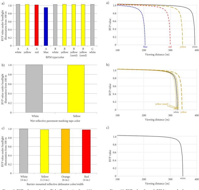
Figure 9. RVP values under headlight illumination from 100 m away for: a – RPMs; b – wet reflective pavement marking tape; c – barrier-mounted reflective delineators
