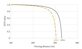
Figure 11. RVP values for each wet reflective pavement marking tape color, as a function of viewing distance
