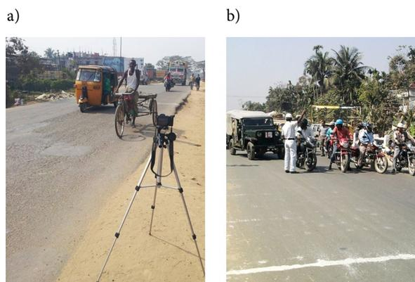
Fig. 3. A view of video photographic survey on the highway section equipped with road markings at: a – uncongested flow conditions; b – congested flow conditions
