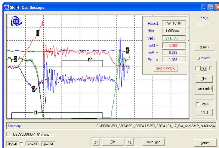
Figure 3. Dynamometer trailer measurement signals: 1 – wheel velocity; 2 – braking torque; 3 – wheel friction force; 4 – wheel normal load
