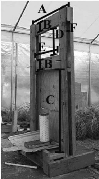
**Fig. 2.** “Car Jack” type briquettes press. Measurements for the press A – 70 cm, B – 15 cm, C – 90 cm, D – 30 cm, E – 55 cm, F – 5 cm (Dahlman, Forst 2001)
