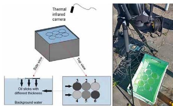
Fig. 1. Diesel detection using infrared camera
