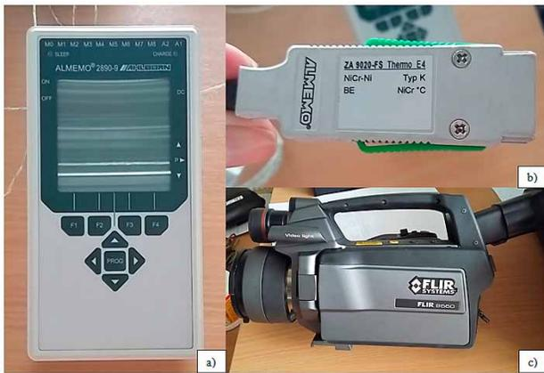
Fig. 2. a) ALMEMO® sensor; b) ALMEMO® connector; c) FLIR camera
