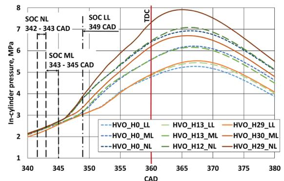
Figure 3. In-cylinder pressure dependence on CAD and position of SOC at various loads and HES with HVO
