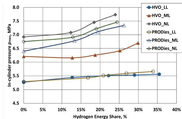
Figure 2. In-cylinder max pressure  $p_{max}$  at Low, Medium and Nominal Loads and HES
