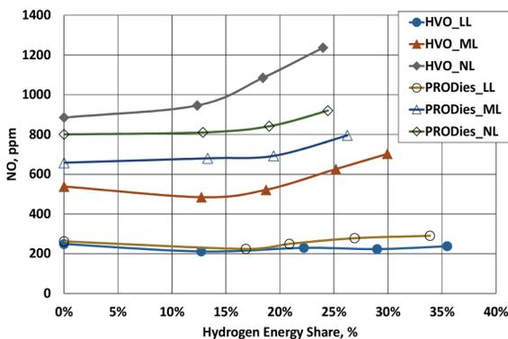
Figure 9. The dependence of NO on the load and HES
