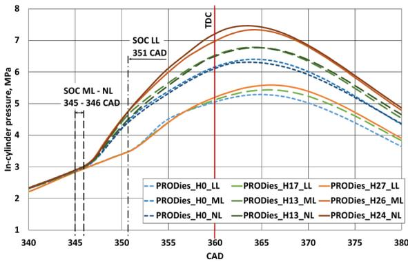
Figure 4. In-cylinder pressure dependence on CAD and position of SOC at various loads and HES with PRO Diesel
