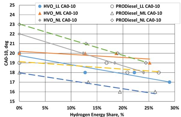
Figure 11. The combustion delay of 0–10% MFB at tested HES of HVO and PRO Diesel
