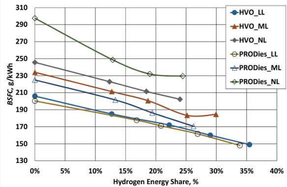
Figure 6. The dependence of BSFC on fuel used, loads and HES
