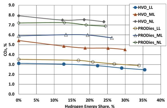
Figure 8. The dependence of CO<sub>2</sub> on fuel used, loads and HES
