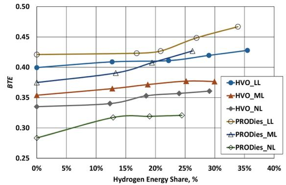
Figure 5. The dependence of BTE on fuel used, loads and HES
