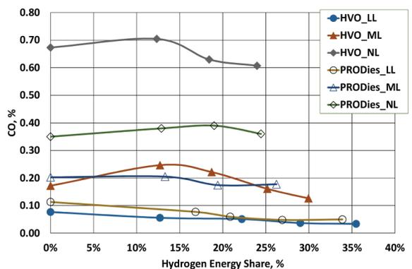
Figure 7. The dependence of CO on fuel used, loads and HES
