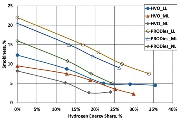
Figure 10. The dependence of smokiness on the load and HES
