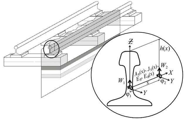
Fig. 2. Parameters assessing rail unevenness
