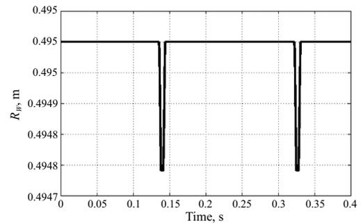
Fig. 4. Changes in radius  $R_w$  of the railway wheelset with the flat ( $L = 100$  m) over time
