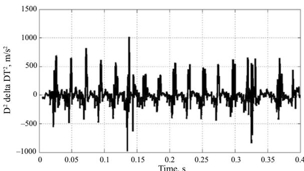
Fig. 9. Changes in the second order time derivative of penetration  $\ddot{\delta}(t)$  over time
