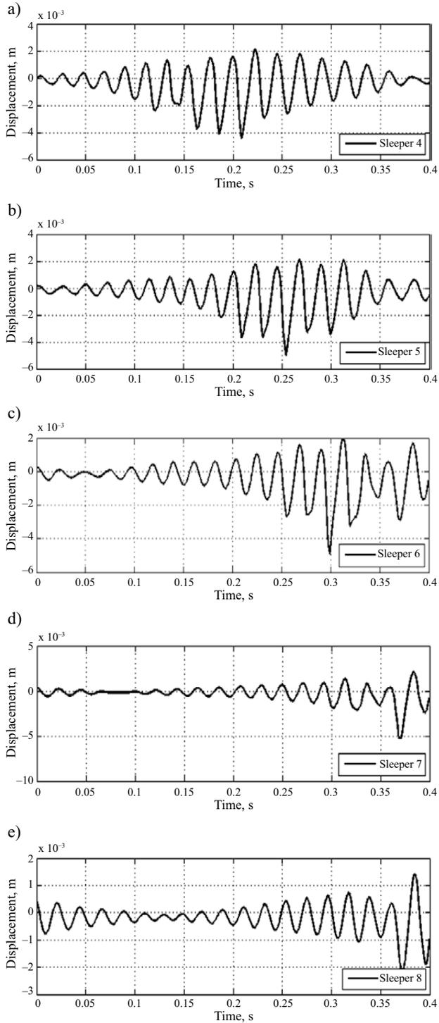
Fig. 5. Displacements of the rail at different nodes of the finite element: (a) 31-th node; (b) 41-th node; (c) 51-th node; (d) 61-th node; (e) 71-th node
