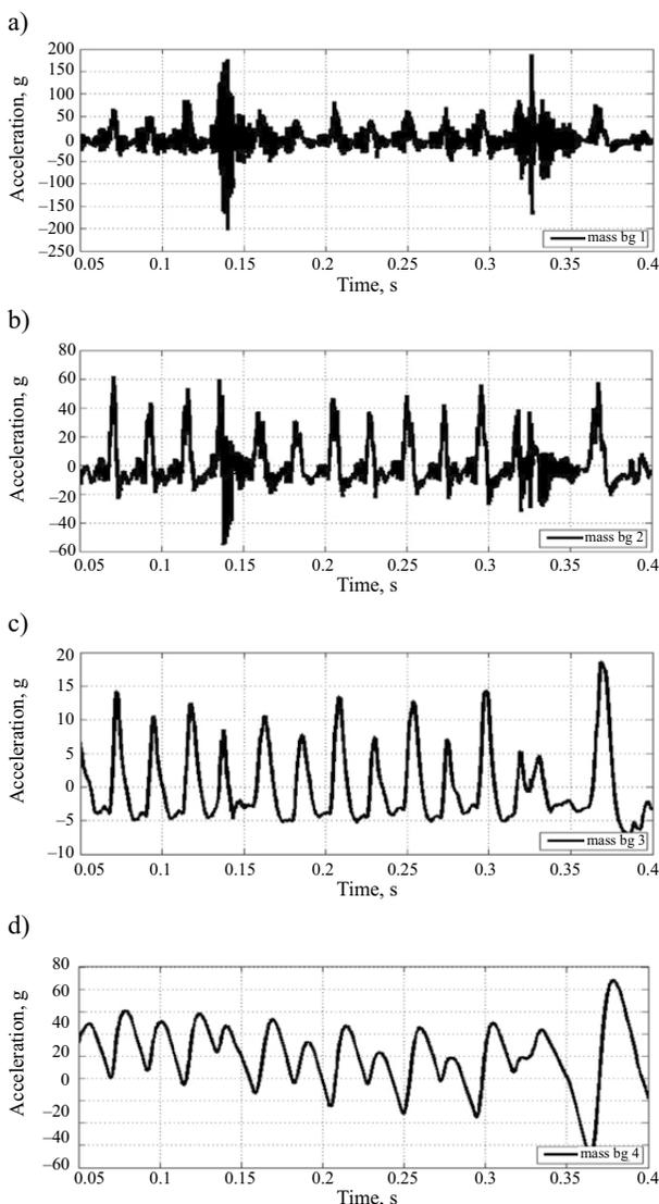
Fig. 11. Changes in the railway vehicle wheelset with vertical accelerations of the flat ( $L = 100$  mm) over time: (a) car body; (b) frame; (c) wheelset; (d) contact mass
