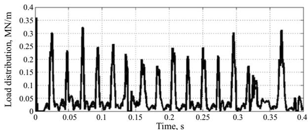
Fig. 10. The dependency of load distribution (9) on the railway vehicle under velocity  $V = 60$  km/h
