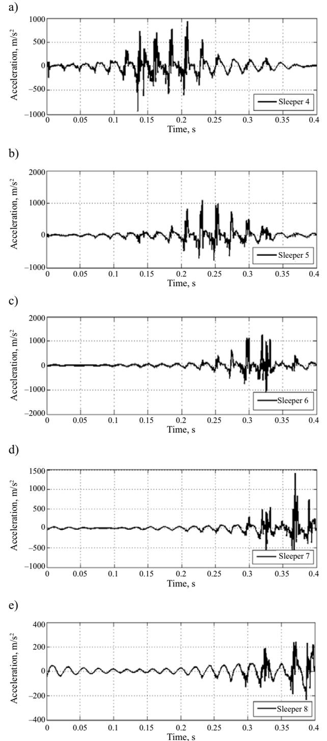
Fig. 6. Accelerations of the rail when the velocity of the train is 60 km/h at different nodes of the finite element: (a) 31-th node; (b) 41-th node; (c) 51-th node; (d) 61-th node; (e) 71-th node
