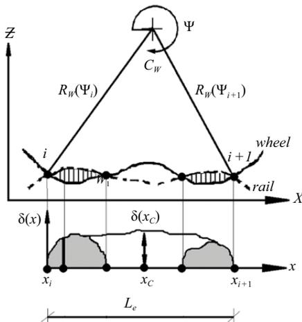
Fig. 3. Geometric parameters of the contact area of the wagon wheel and the rail
