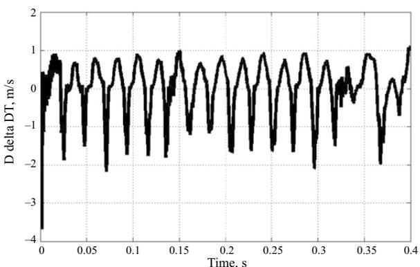
Fig. 8. Changes in the time derivative of penetration  $\dot{\delta}(t)$  over time
