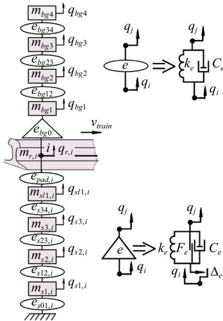
Fig. 1. Dynamic model of the system *Railway Vehicle Wheel–Track*: (a) scheme; (b) nonlinear elastic–damping discrete element, (c) linear elastic–damping discrete element
