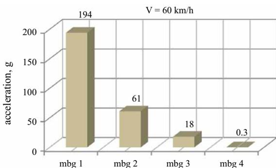
Fig. 12. A comparison of vertical accelerations of the mass of the wagon
