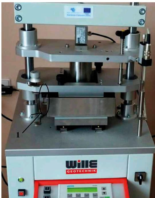
Fig. 3. Direct shear apparatus. 1 – external horizontal displacement transducer
