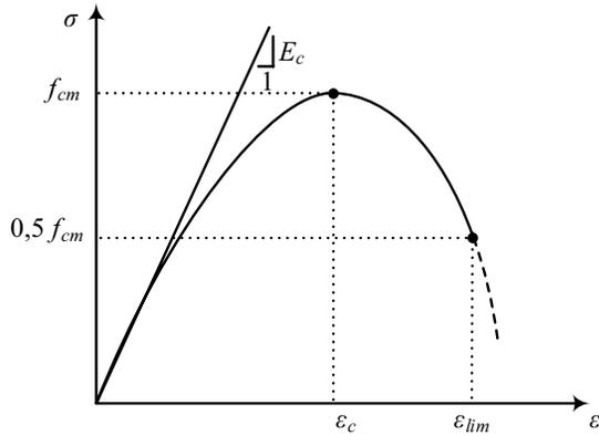
Fig. 1. Static stress-strain relationship for concrete in compression
