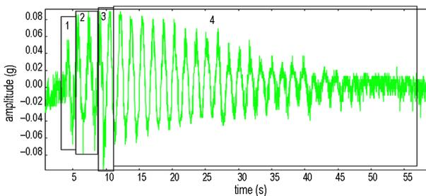
Fig. 9. Manually operated crane with empty container accelerations
