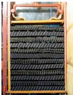
Fig. 2. Structured packing block made in form of particular short layers
