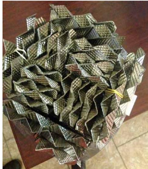
Fig. 15. Proposed packing CUB
