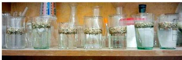
Fig. 3. Water sorption capacity determination test
