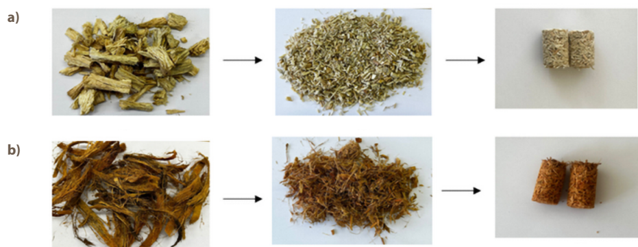
Figure 1. Preparation of samples from raw materials to trimmed materials and mold specimen steps: a) sugarcane fiber; b) coconut fiber
