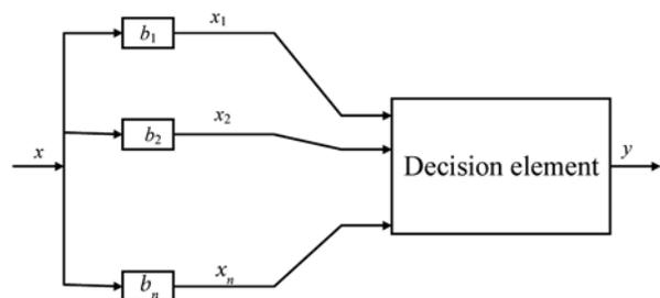
Fig. 1. McCulloch-Pitts artificial neuron functional scheme
