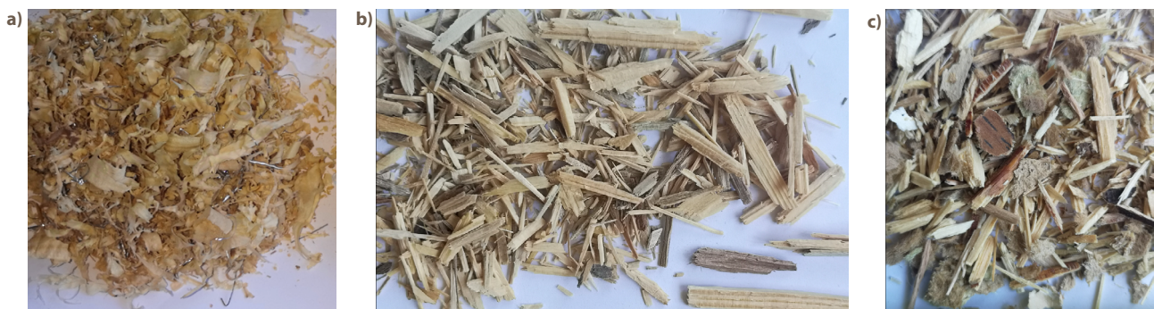
Figure 1. Raw wood waste: a) door production (DW) industry; b) wooden packaging (W); c) furniture and construction demolition (PLY) industry
