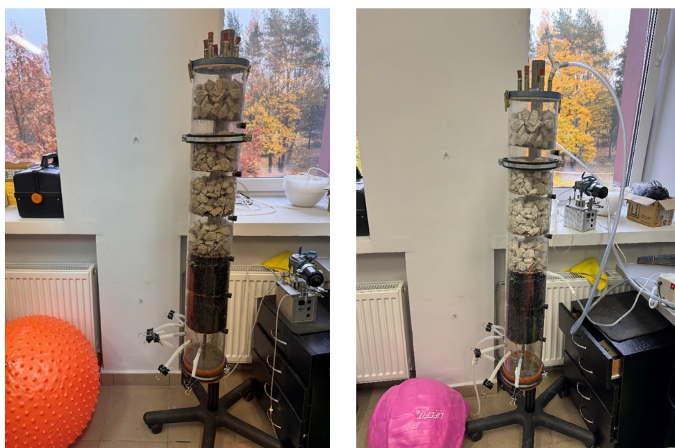
Figure 1. Lab-scale biofilter structure and main components
