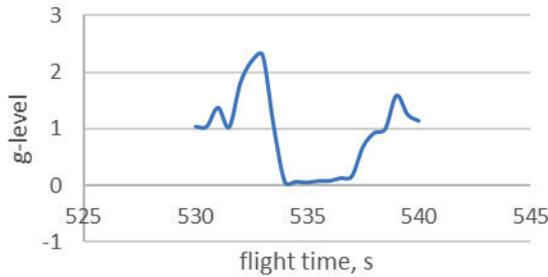
Fig. 4. Typical g- level test result during simulator parabola flight
