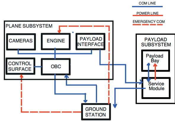
Fig. 3. Plane subsystems scheme
