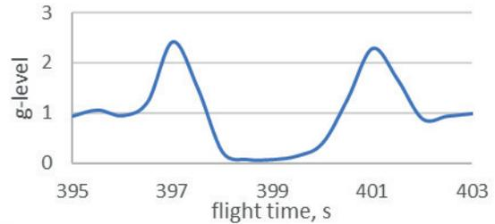
Fig. 6. Typical g- level test result during real parabola fight
