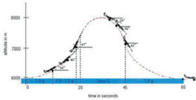
Fig. 1. Parabolic flight path
