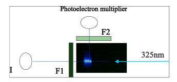
**Fig 1.** Experimental setup. He-Cd laser light of 325 nm falls on a sample in a kvarz cuvette. UV light is absorbed and blue visible light emitted by a sample. Transmission and luminescence are measured simultaneously. Colour optical glass filters used to separate the UV and VIS light components were F1-  $V\Phi C6$  (transmit above 280 nm and below 420 nm) and F2- EC7 (transmit above 340 nm)
