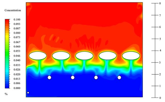
Figure 7. The diagram of distribution of the CO<sub>2</sub> concentration within the capacity of winter garden
