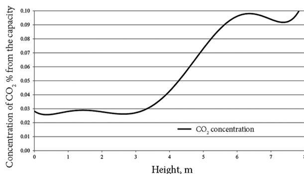
Figure 9. Modification of the concentration of  $\text{CO}_2$  at the height of a winter garden
