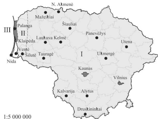
Fig. 5. The map of basic reference wind speeds  $v_{ref,d}$  specified in the design code STR 2.05.04:2003 (see also Table 2)
