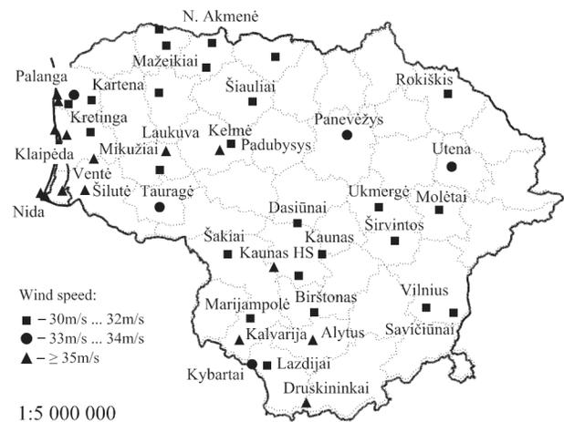
**Fig. 1.** Map showing the network of Lithuanian weather stations with 10-min wind speeds of at least 30 m/s recorded in 1962–2005 (the geographic coordinates of the stations were provided by Lithuanian Hydrometeorological Service, <http://www.meteo.lt/>)
