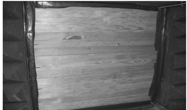
Fig. 6. A log wall, 15 cm wide, assembled in the noise suppression chamber and covered with cladding, 2 cm wide
