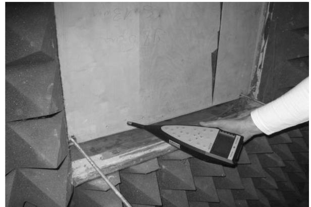
**Fig. 2.** Checking noise emission through spaces that emerged in the structure
