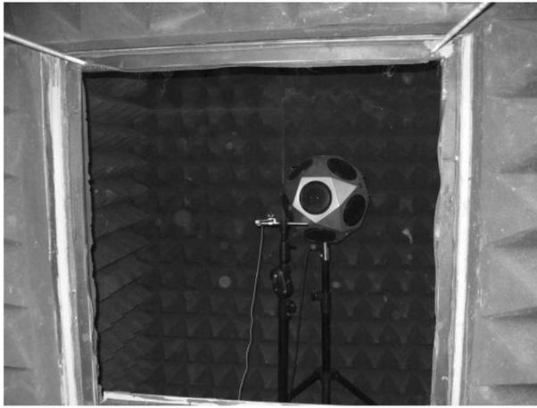
**Fig. 1.** Noise suppression chamber and a "window" wherein the specimen is mounted
