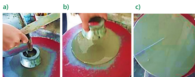
Figure 12. Consistency test steps: a) filling of the conical trunk; b) removal of the formwork vertically; c) verification of the spreading measure
