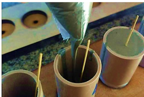
Figure 15. Procedure for molding the specimens for the pullout test
